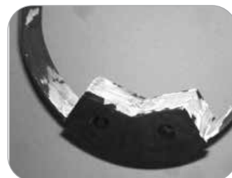
Additional sealant applied to V-Block saddle joint between the two saddle halves. (Chilled water below 50°F).
